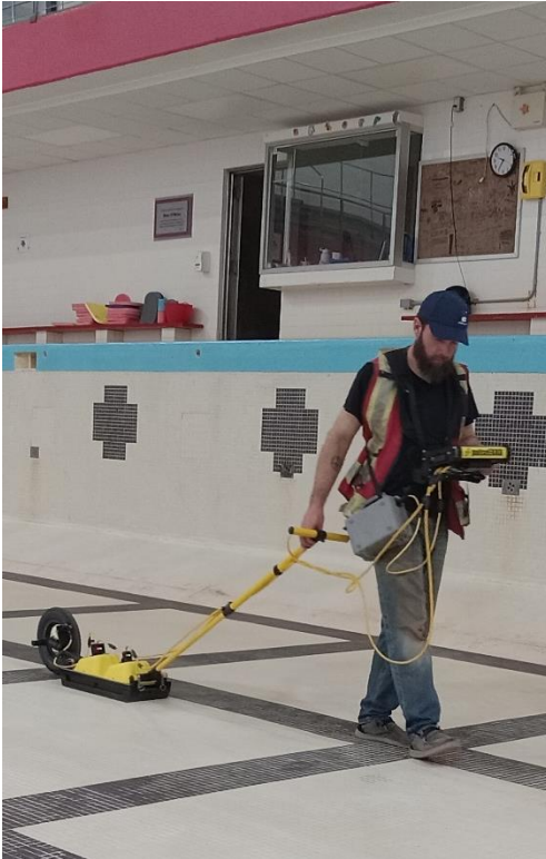
Figure 2.1.1 – Pulse Ekko tow-behind configuration with the 500MHz antenna.
